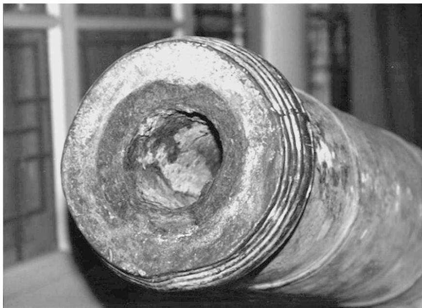
Figure 30. The muzzle of the gun in Figure 29. Note that it is iron on the inside
