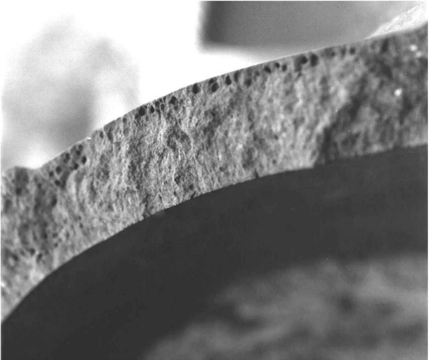
Figure 14. Detail of the fracture of the bell shown in Figure 13 (photo by author).
