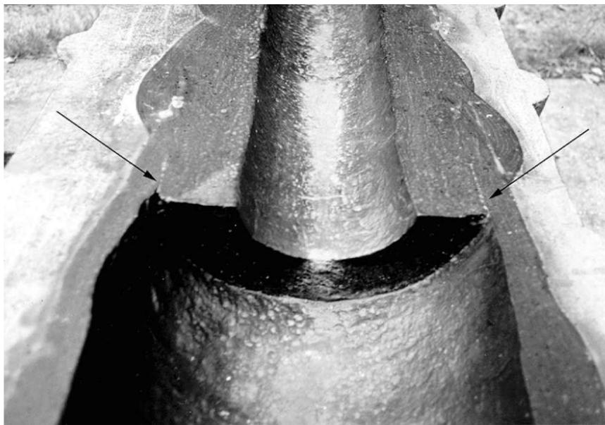
Figure 32. Detail of the gun on the left in Figure 31. The arrows indicate the boundary between two layers of iron (photo by author).
