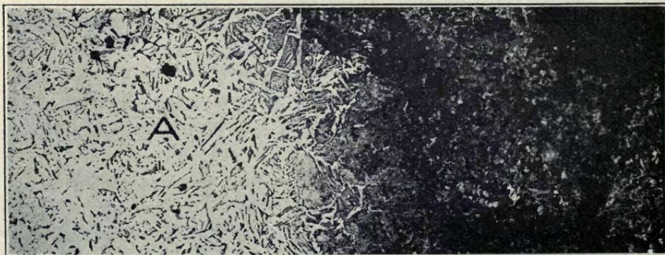
Fig. 121—Ineffective hard weld of malleable casting using ingot iron wire and
