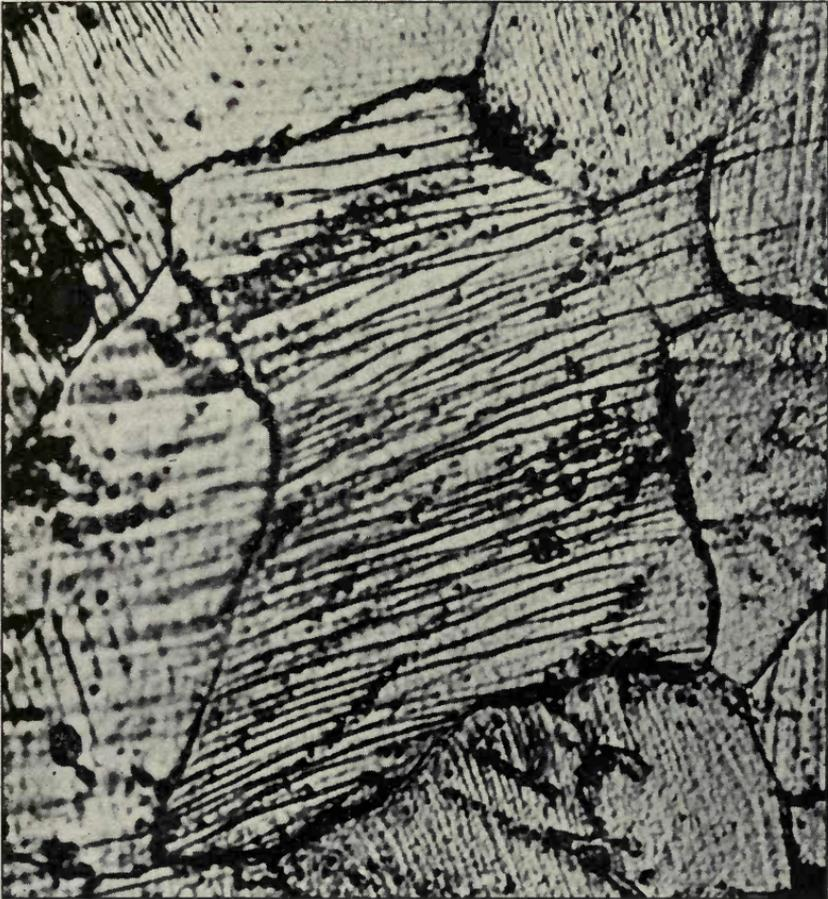
Fig. 164.—Slip bands in ferrite of malleable iron
