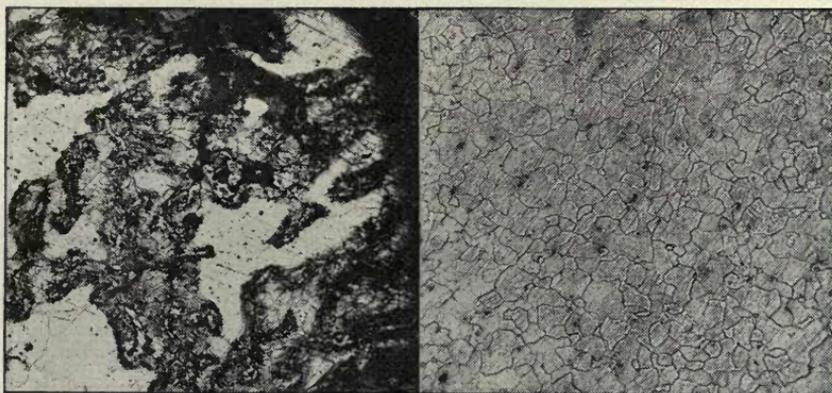
Fig. 117—(left)—Cementite persisting near a shrink. The metal in porous areas is somewhat oxidized. Fig. 118—(right)
