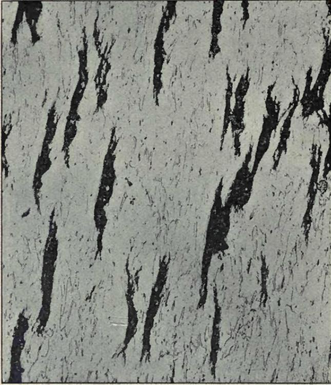
Fig. 169.—Plastic deformation of malleable in compression
