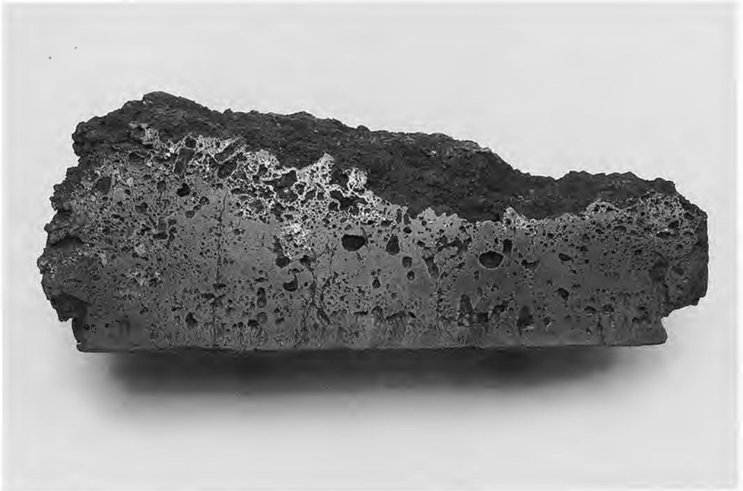
Fig. 7. Section of a slag "bottom" from the Caldwell forge site. Columnar fayalite crystals extend upward from the flat bottom surface. Unlike the "skulls," the slag in the "bottom" is free of iron particles, although there are iron rims around some of the pieces of charcoal near the top of the specimen. The length of the section is 230 mm. (Specimen collected by Gordon Pollard; photograph by William Sacco)
