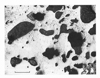
Polished and etched section through a Danish clot (Vejle Museum nr.22072). Phosphorusrich iron (white), alternate with slag inclusions (grey), and voids and corrosion products (black). Scale bar 0.5 mm.
