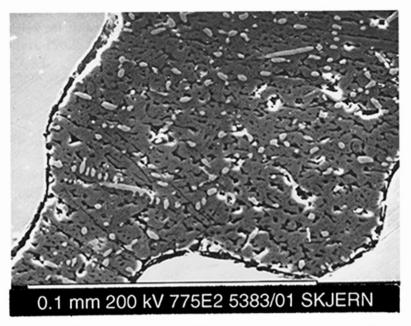
Polished section through a Danish clot (Skjern Museum, three-fingered, 4.8 kg). The slag consists of major phosphofayalite (grey, 1-2 wt% P) and minor wüstite (light grey dendrites) and glass matrix (black, 10-12 wt% P).
