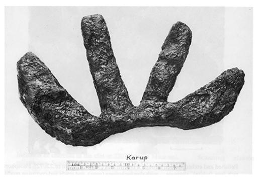
Four-fingered clot (Danish: klode) found in 1920 near Karup, Jutland. Now in Vejle Museum (Karup I, nr.963x1). With a volume of 1.9 l and a weight of 8.2 kg, the specific gravity is only 4.3g/cm³. Metallographic examination shows that the material is 50 vol% iron and 50 vol% slag. Before corrosion altered the clot somewhat, the weight must have been about 10 kg and the spec. grav. about 5.2 g/cm³.
