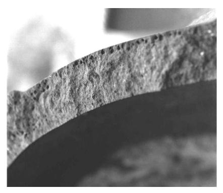
Figure 14. Detail of the fracture of the bell shown in Figure 13 (photo by author).
