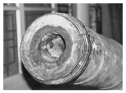
Figure 30. The muzzle of the gun in Figure 29. Note that it is iron on the inside and bronze on the outside (photo by author).
