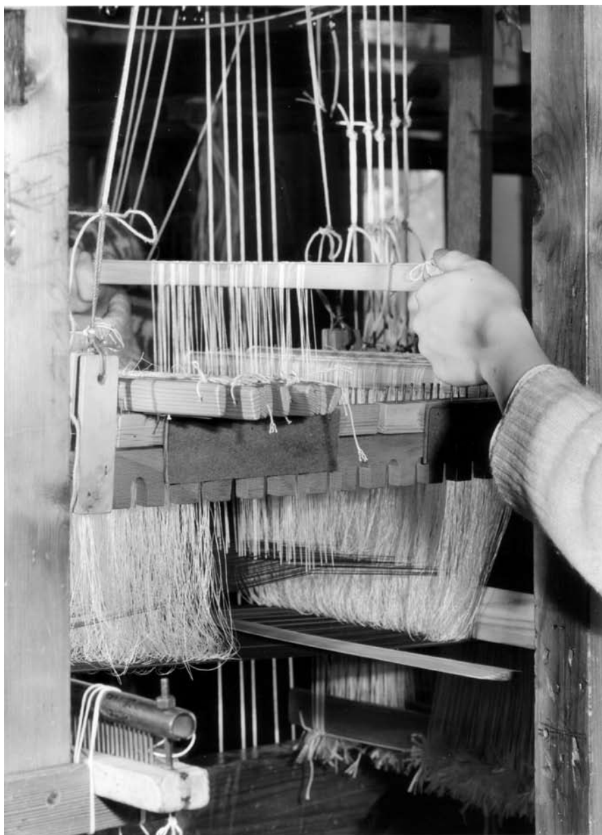
Figure 63 Two pattern heddle rods are lifted for the pattern weft; the shed is cleared up by means of a flat stick.
