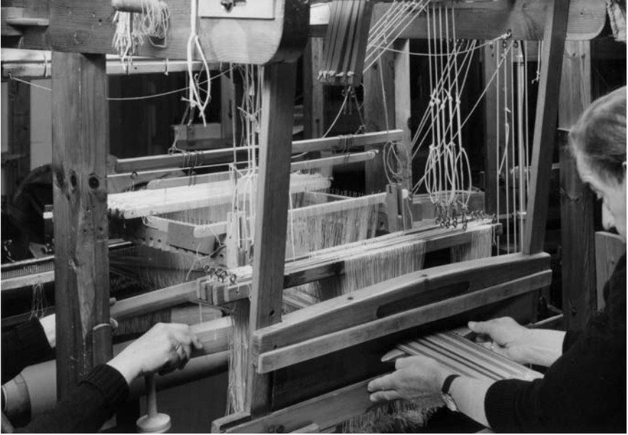
Figure 58 The loom set up with a three-coloured silk. Note our device for lifting one pattern heddle rod. One flat stick is placed below the lifted rod, the other stick helps to open the pattern shed to the weaver.
