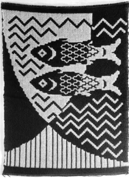
Figure 186 The face side of our example of double cloth woven with a working drawing fastened below the warp.
