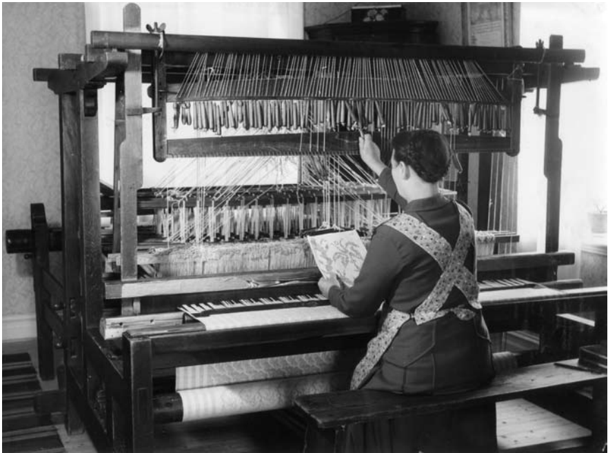
Figure 220 A Swedish damask weaver, Maria Andersson, working with one hundred pattern shafts, photographed in 1950. The loom was built for her mother in the late 19th century by a country carpenter after Ekenmark's descriptions.
