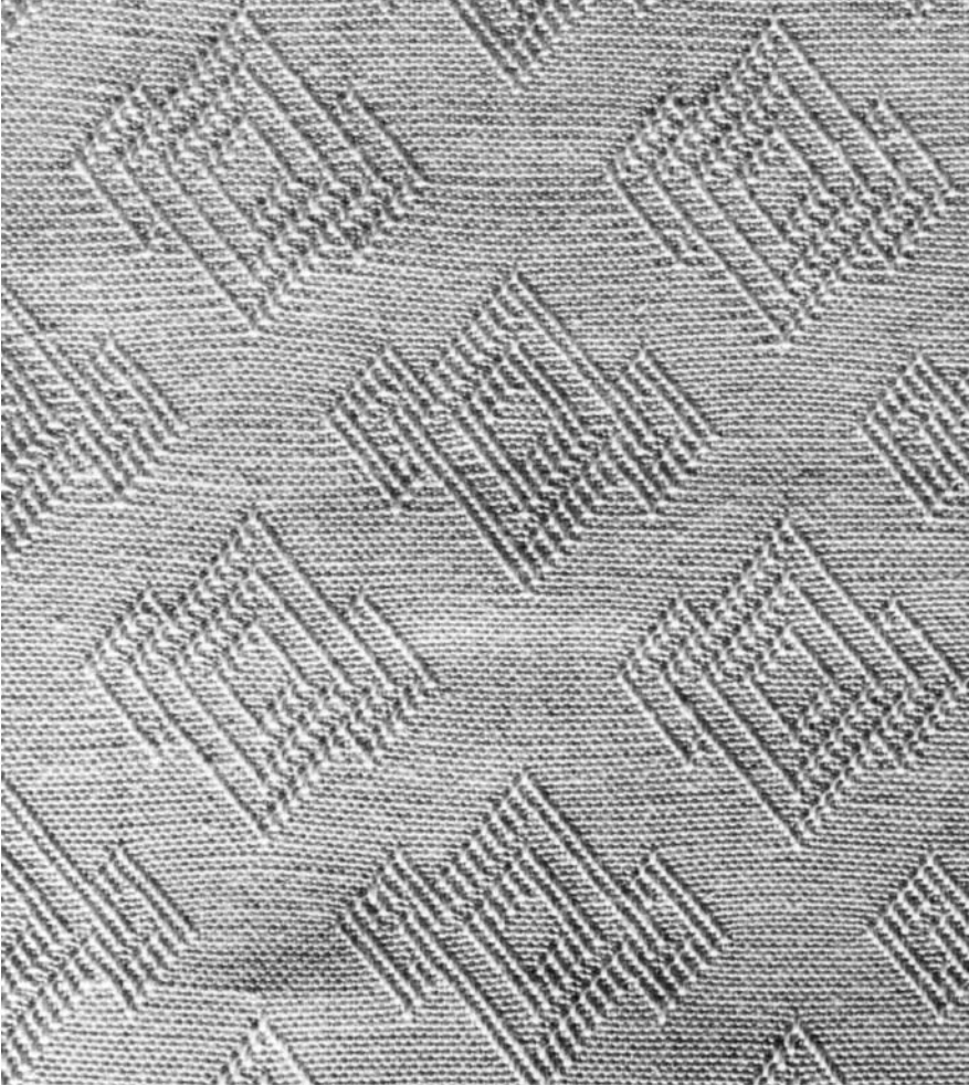
Figure 17 Monochrome patterned silk woven according to the draft of Figure 16. Note the effect of twill direction, following the contour on two sides and opposing it on two sides.
