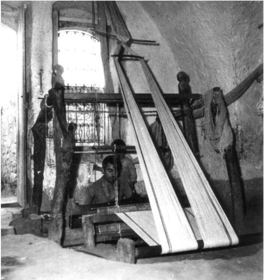
Figure 242 Horizontal loom with the treadles in a pit. The length of warp is fastened on the wall behind the weaver. Azaz, North Syria, 1961.
