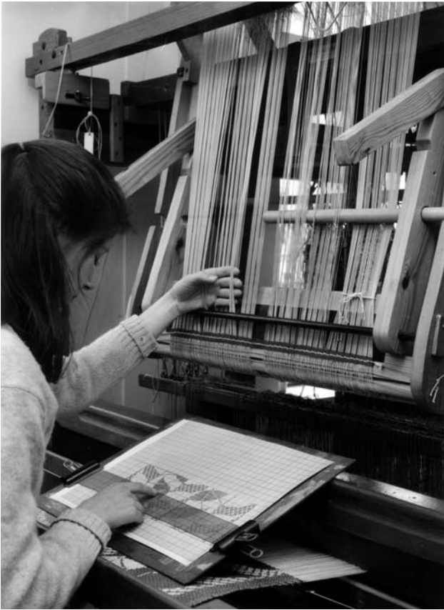
Figure 264 A pattern is counted up following the design on ruled paper. Each row is taken onto the round rod in the shed lifter.
