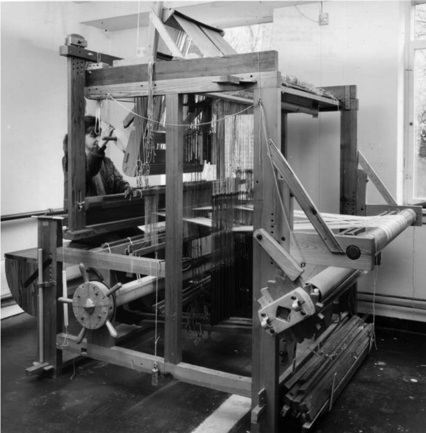
Figure 259 Our drawloom attachment mounted onto a counter-march loom. The shed lifter is here pulled forward to open a pattern shed. Extended space for the warp is obtained by inserting the back beam between two longer boards. Side frames are raised to give space for counter-weights for shafts.
