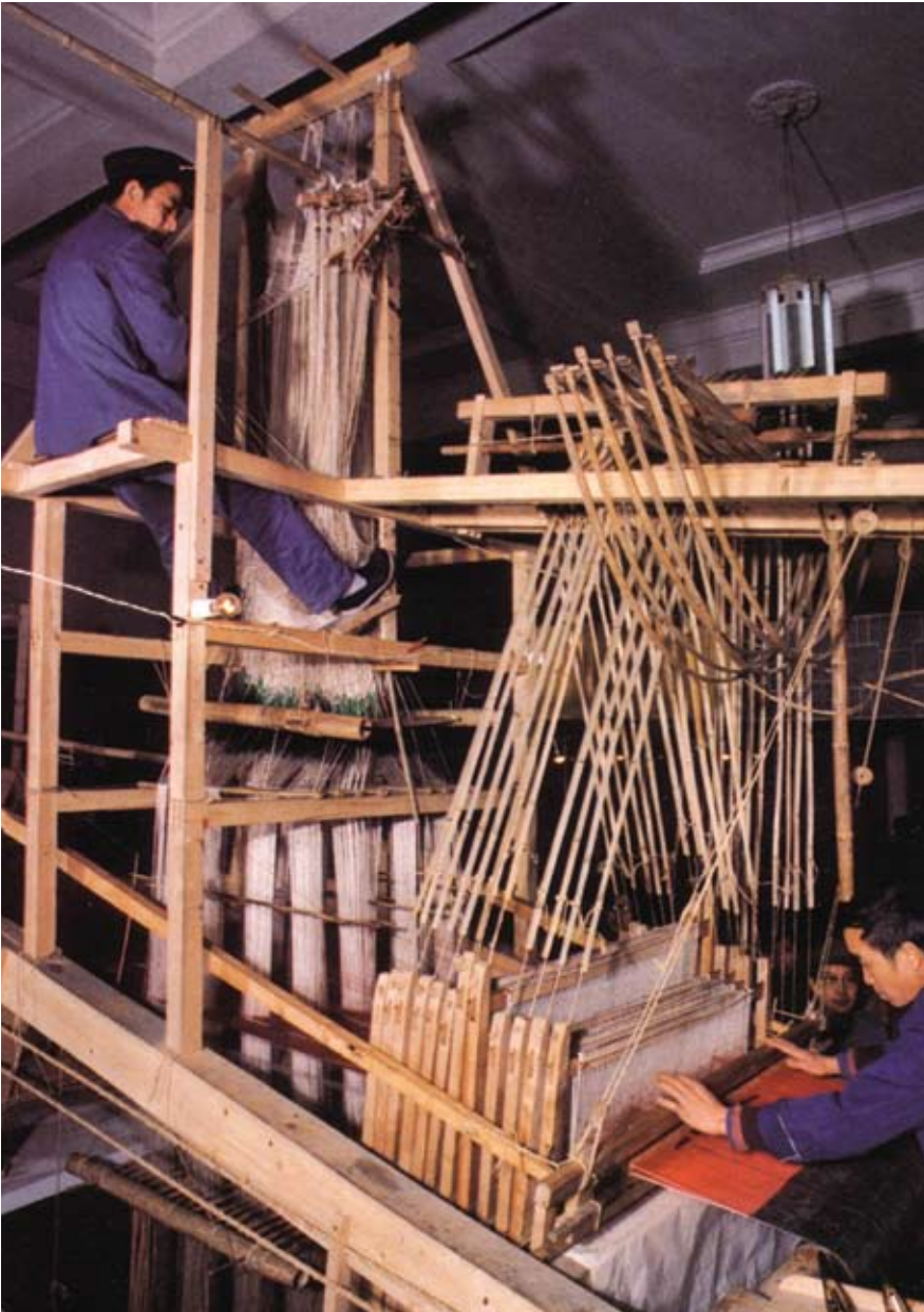
Figure 246 A modern working reconstruction of a Chinese drawloom (exhibition catalogue from Ontario Science Centre, 1982). Note that the six depression shafts, nearest to the weaver, are supplied with bows to bring up the shafts to their former position when they are released. In this case the shafts are fastened to the horizontal upper rods (bow strings) and the lower bows help to straighten out the upper rods.
