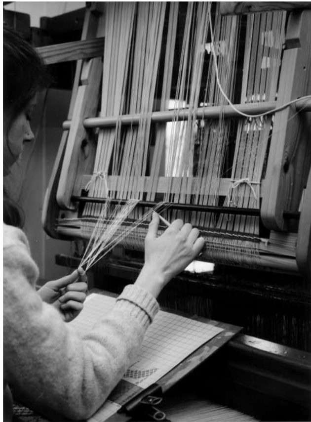
Figure 265 The making of lashes. Note the thin string at the right. A loop is pulled forward between lifted harness cords. Each of the lashes is secured by a cord (gavacine) knotted onto the guide momentarily hung up on the right.
