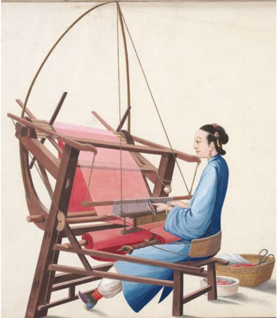
Figure 268 Watercolour drawing showing the slanting Chinese loom for weaving silk tabby. The shaft is supplied with open heddle loops, type A. Note the thin round rod placed into the heddles. The drawing belongs to The Royal Library, Copenhagen, Department of Manuscripts (New Royal Coll. 346 a).
