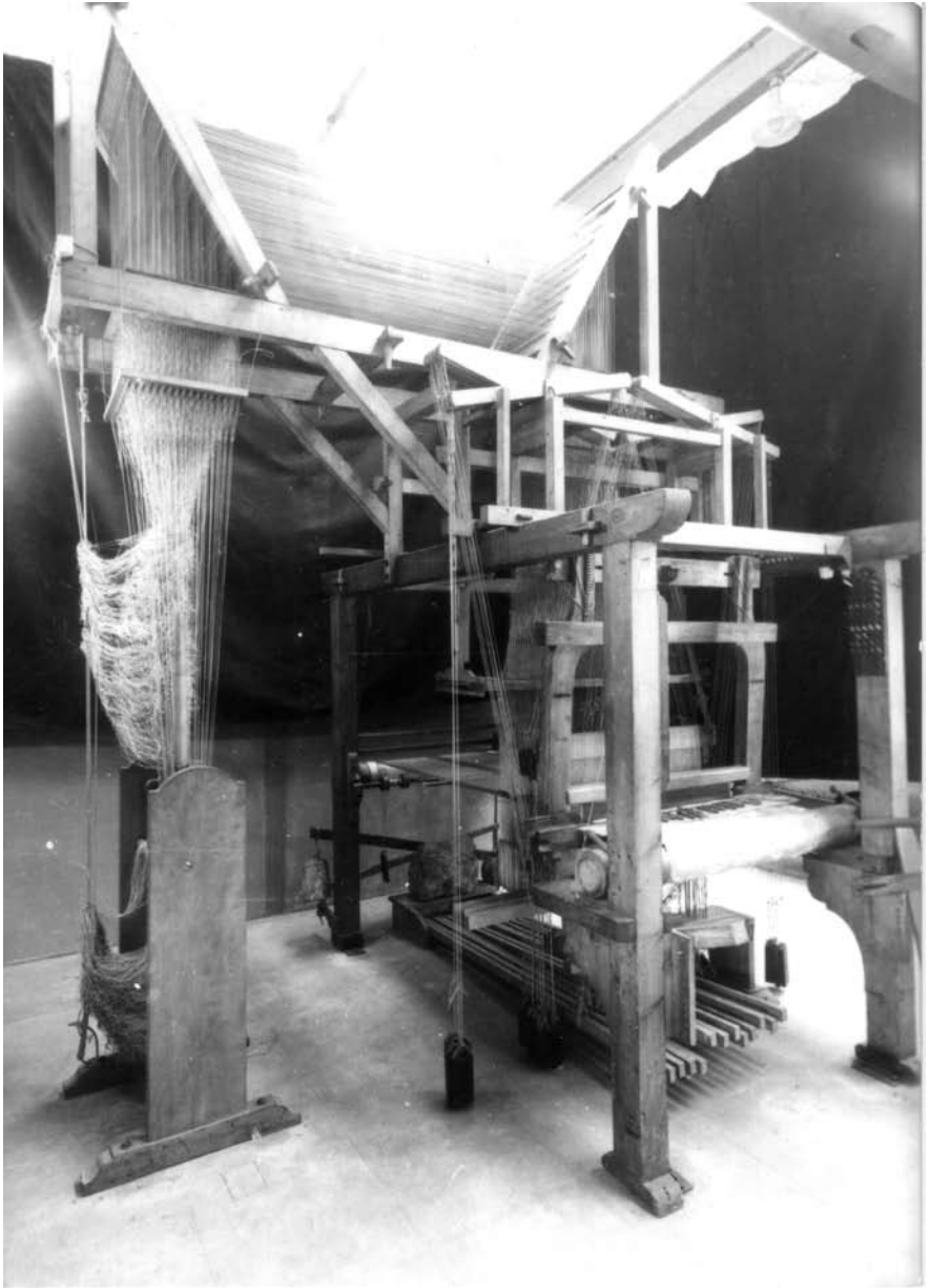
Figure 253 Philippe de Lasalle's drawloom reconstructed by F. Guicherd according to descriptions from the 18th century. This is an example of the other type of drawloom with two oppositely slanting pulley boxes. The loom is now on exhibition in 'la Maison des Canuts', Lyon, together with other old looms and implements in working order. The photograph belongs to École de Tissage, Lyon, reproduced by kind permission from M. Vial.
