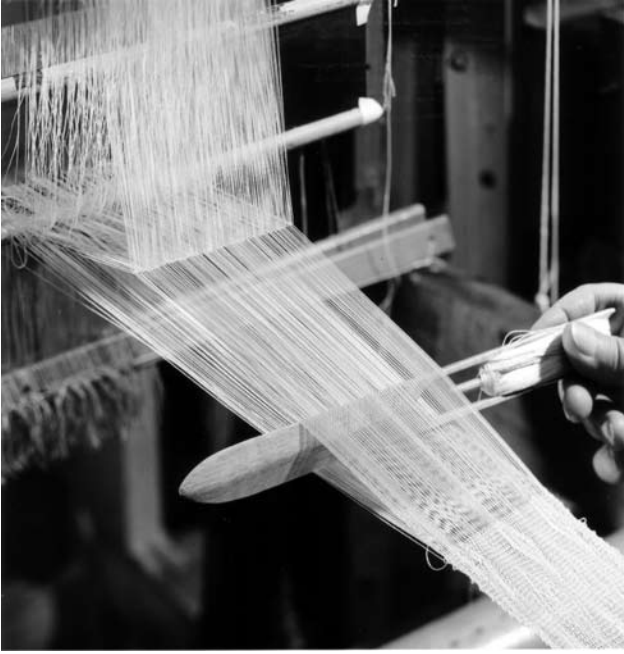
← Figure 40 Doup shaft B is lifted and the little flat shuttle is placed in the shed.
