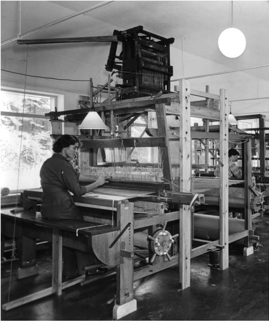
Figure 257 A Jacquard loom in our workshop set up for damask tablecloths. Note that the weaver has pressed down the long treadle which lifts the current row of pattern. At the same time the pivoting frame with the prism is pressed outward and a new card for the next row is turned out. Five shafts and five treadles are used for the satin weave.
