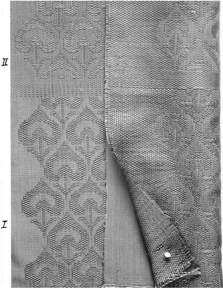
Figure 124 The woven samples I and II are shown with the face side up at the left and folded over to show the reverse side at the right. Note in sample I (lower left) the plain tabby ground and compare this with the ground in sample II.
