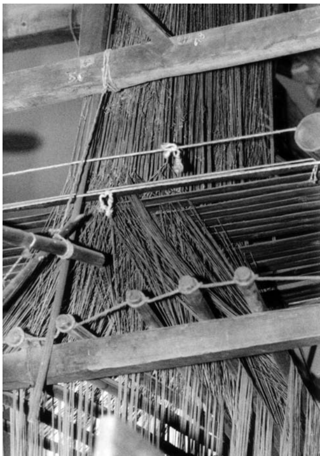
Figure 248 A detail of the drawloom in the Museum of Chinese History, Beijing, which shows how repeats of pattern units are obtained.
